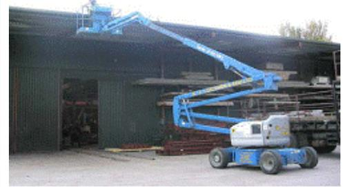
*Using a MEWP to clean a gutter*
